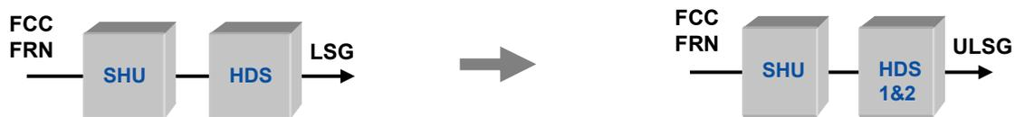
The most common post-treatment scheme is the Prime-G+ 1<sup>st</sup> Step followed by a single HDS section. Revamping this scheme to include a second HDS reaction section offers the maximum octane retention, minimum hydrogen consumption and increased cycle.
