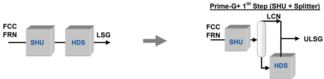
Another route for revamp of the basic post-treater is to add a second HDS reaction section. Treating the FCC naphtha in two stages reduces octane loss and hydrogen consumption while increasing the cycle length.
