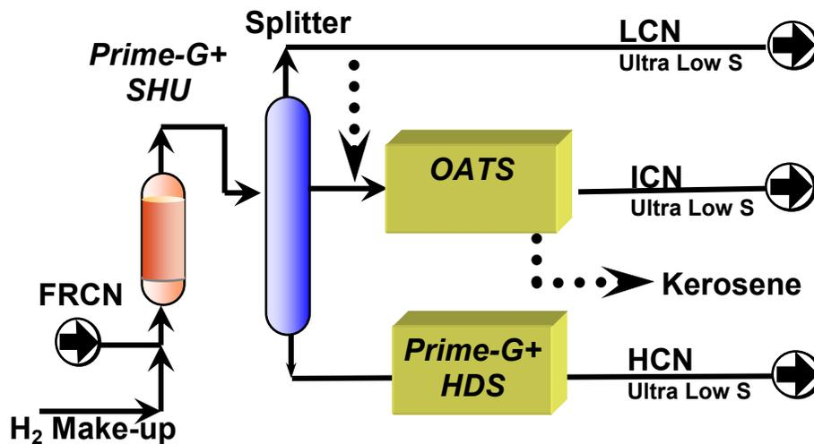
An additional benefit of the OATS technology is an olefin shift. Light olefins dimerize to form a C<sub>10</sub>-C<sub>12</sub> product which shifts light gasoline to the distillate pool. The reduction of C<sub>5</sub> and C<sub>6</sub> olefins in the FCC gasoline also improves the RVP. Isomerization of olefins that do not dimerize makes the process octane neutral.
