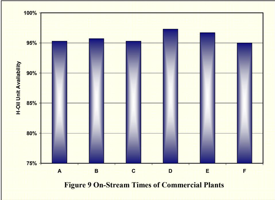
The plot shown in Figure 9 reflects Unit Availability for 6 H-Oil<sup>®</sup> Commercial Operating Plants. Unit Availability is defined as the actual on-stream time less planned turnarounds (typically occurs once every 3 to 6 years) and outages due to external factors (i.e. hurricane on the Gulf Coast).
