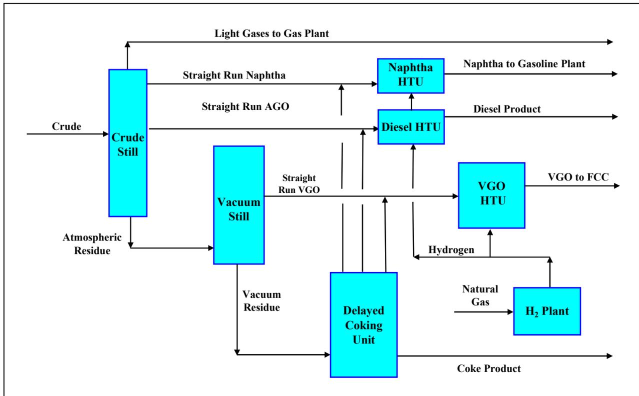
Two expansion configurations were investigated for this study. The first case (Case 1) adds an additional 100,000 bpsd of Arabian Heavy Crude and duplicates the existing 27,200 bpsd Delayed Coker. The expansion brings the total crude throughput to 200,000 bpsd. The battery limits of Axens study is shown in Exhibit 1 and includes the associated offsite and utilities. It does not include the FCC Unit or the post FCC hydrotreater (i.e. Prime G+).
